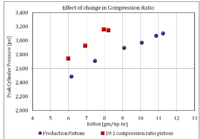
**Figure 20 - 19:1 Wide/Shallow Piston, PCP vs bsNOx**
