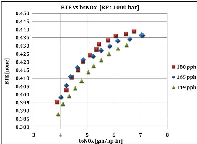
**Figure 27 - 19:1 Scaled Production Piston BTE vs bsNOx, 1000 bar Rail Pressure**
