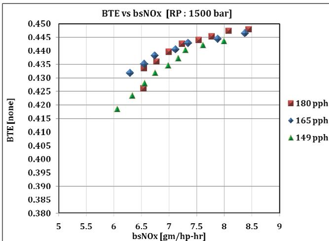
**Figure 28 - 19:1 Scaled Production Piston BTE vs bsNOx, 1500 bar Rail Pressure**
