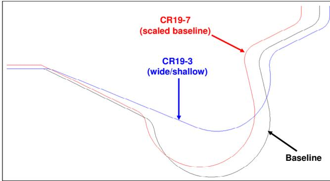
**Figure 1 - Piston Geometries**
