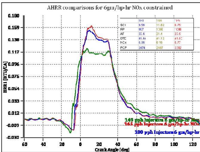
**Figure 18 - Apparent Heat Release at 6 g/hp-hr bsNOx 149, 165, & 180 pph Injectors**
