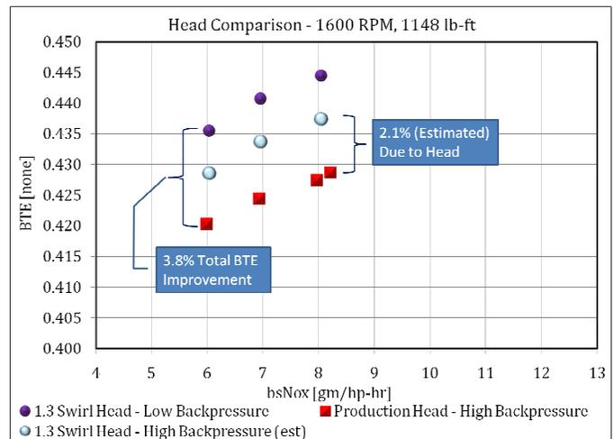
**Figure 25 - BTE Comparison, 1600 RPM 1148 lb-ft
