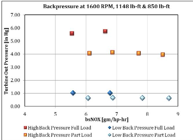
**Figure 21 - Backpressure at 1600 RPM 1148 lb-ft & 850 lb-ft**
