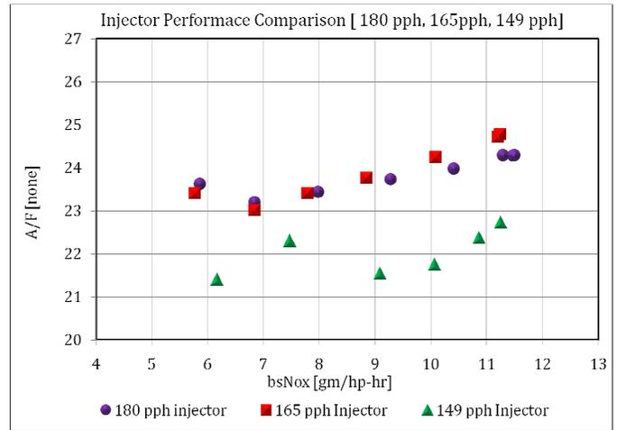
Figure 15 - Injector Comparison, A/F vs bsNOx
