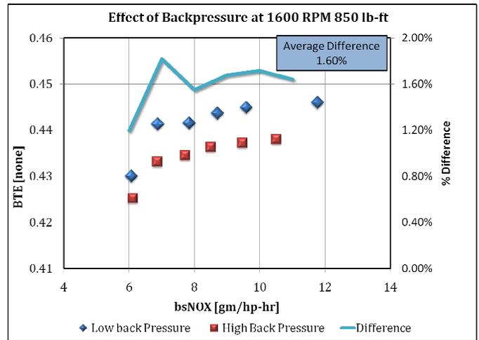
**Figure 23 - Effect of Backpressure on BTE 1600 RPM, 850 lb-ft**
