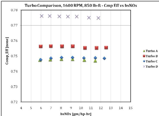
Figure 31 - Compressor Efficiency vs bsNOx
