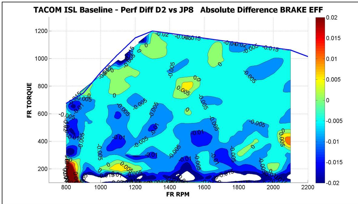
Figure 8 – Change in Brake Thermal Efficiency Due to Operation on JP-8
