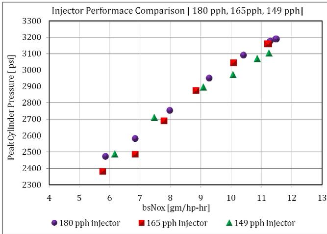
Figure 14 - Injector Comparison Peak Cylinder Pressure vs bsNOx
