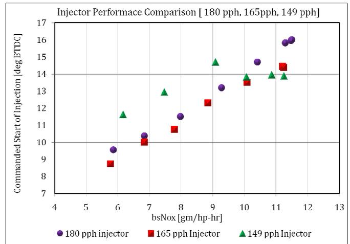
Figure 16 - Injector Comparison Commanded Start of Injection vs bsNOx
