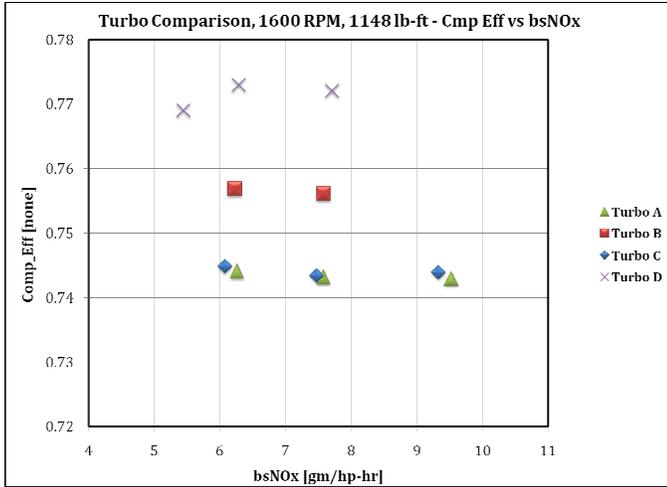
Figure 30 - Compressor Efficiency vs bsNOx
