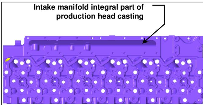
**Figure 2 - Production Head with Intake Manifold**
