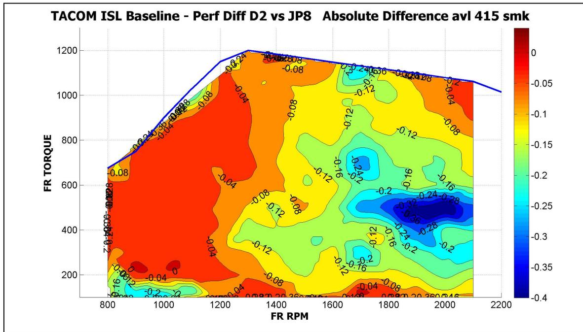
Figure 10 - Performance with JP-8 Compared to Diesel, Difference in Smoke (FSN)
