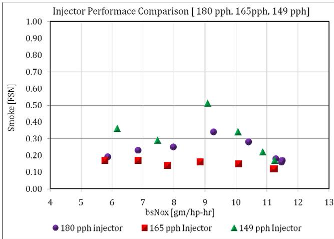
Figure 13 - Injector Comparison, Smoke vs bsNOx
