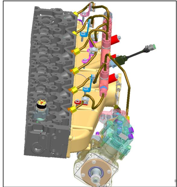
**Figure 3 - Modified head with bolt on intake manifold**
