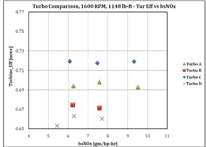
Figure 32 - Turbine Efficiency vs bsNOx
