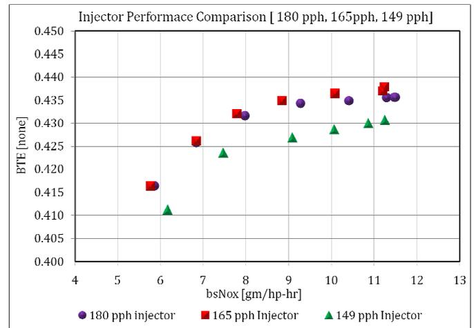
**Figure 12 - Injector Comparison, BTE vs bsNOx**
