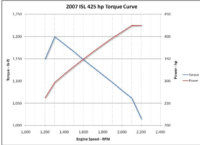
**Figure 4 - 2007 ISL 425 hp Torque Curve**
