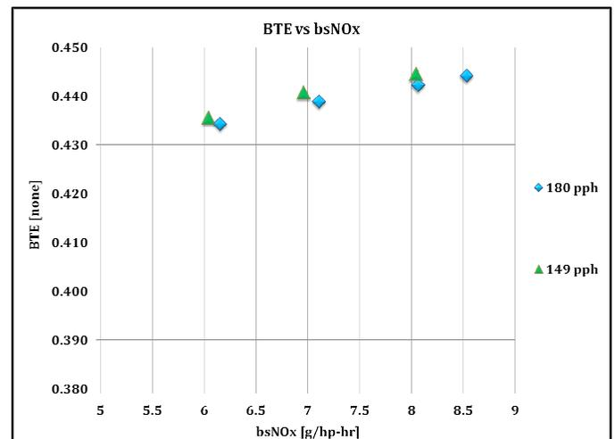
**Figure 29 - 19:1 Wide/Shallow Piston, BTE vs bsNOx**
