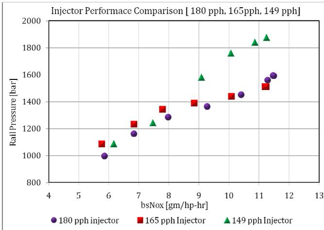
**Figure 17 - Injector Comparison, Rail Pressure vs bsNOx**
