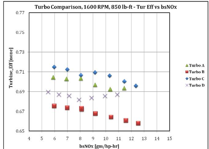
Figure 33 - Turbine Efficiency vs bsNOx
