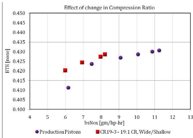
**Figure 19 - 19:1 Wide/Shallow Piston, BTE vs bsNOx**
