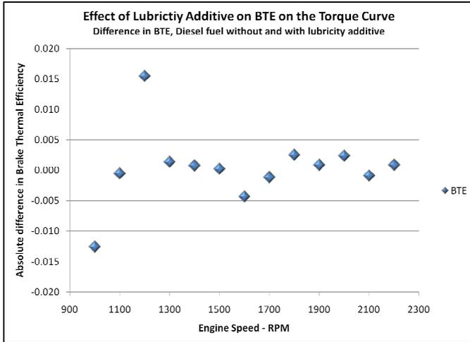
**Figure 6 - Difference in Brake Thermal Efficiency Diesel fuel with and without lubricity additive**
