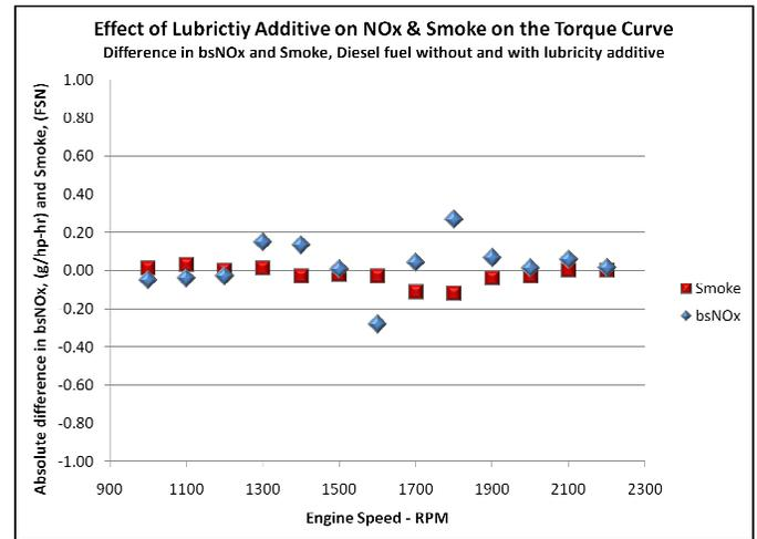
**Figure 5 - Difference in bsNOx and Smoke Diesel fuel with and without lubricity additive**
