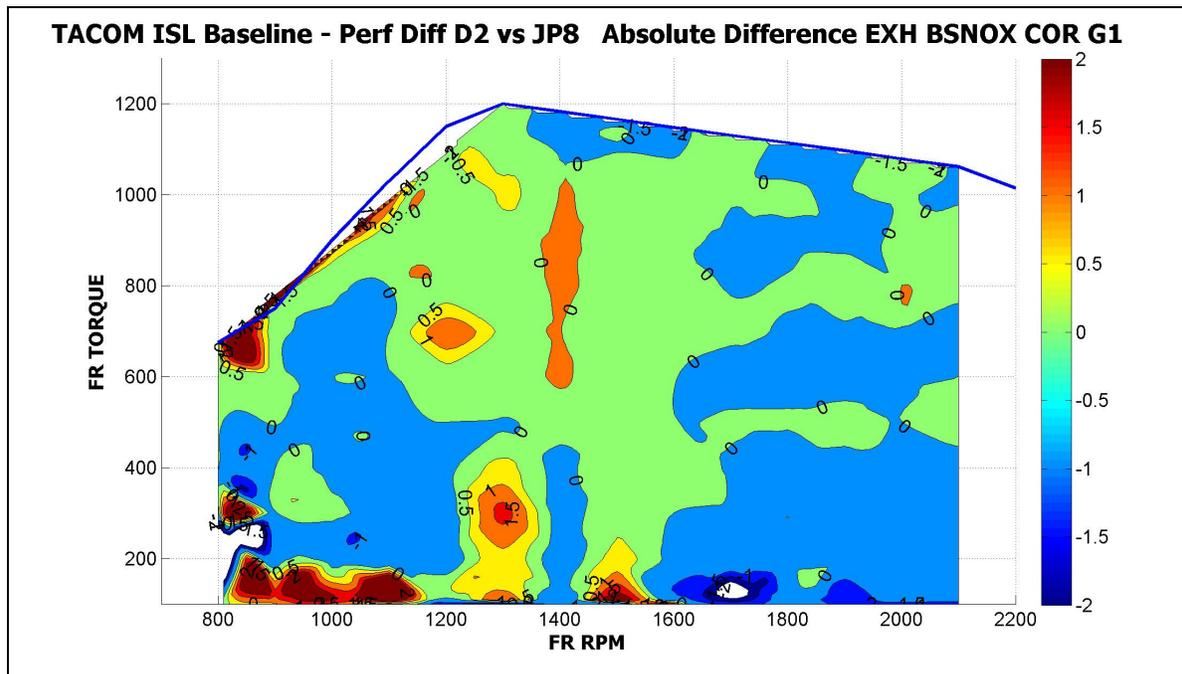
Figure 9 - Change in bsNOx (g/hp-hr) Due to Operation on JP-8
