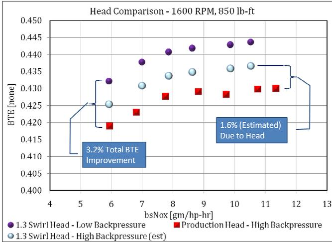
**Figure 26 - BTE Comparison, 1600 RPM 850 lb-ft Production Head & Modified Head**
