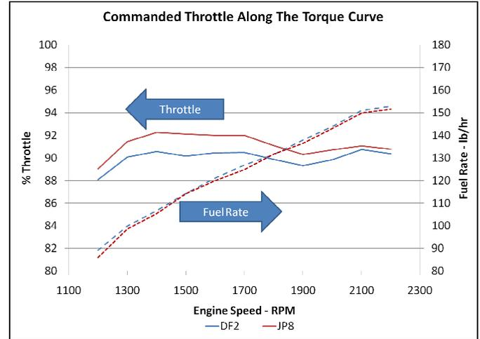
**Figure 7 - Fuel Rate & Commanded Throttle Along the Torque Curve**
