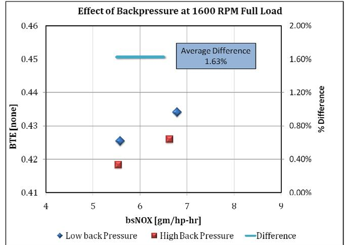
**Figure 22 - Effect of Backpressure on BTE 1600 RPM, 1148 lb-ft**
